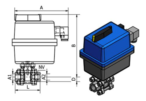
= - Connecting A2 = G 1 1/2" = - D = 40 = - L = 104 = - Max. Operating Pressure = 25 bar = - NV = 58
